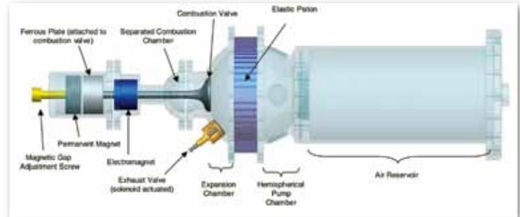
**Project Goal:** Develop a compact high energy density pneumatic power supply applicable to untethered fluid-power applications that is an order of magnitude more power dense than existing technologies. This will be achieved by designing, building and testing a free-piston engine utilizing spark-ignited fuel that is specifically load matched to the task of compressing air.
