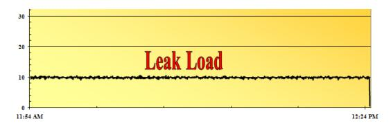
This is an example of the leak load on a case packer that had been in operation. Several leaks were found on the machine – worn cylinders, broken fittings, etc. The static flow seen on the chart is indicative of leaks and wasted air. While 10 CFM may not seem like much, it is over 35% of this case packers average flow which is normally 27. 9 CFM.
