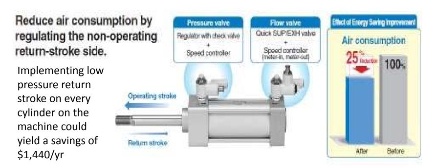
A typical savings of up to 25% per machine can be achieved. Image courtesy of SMC. SMC model ASR.
