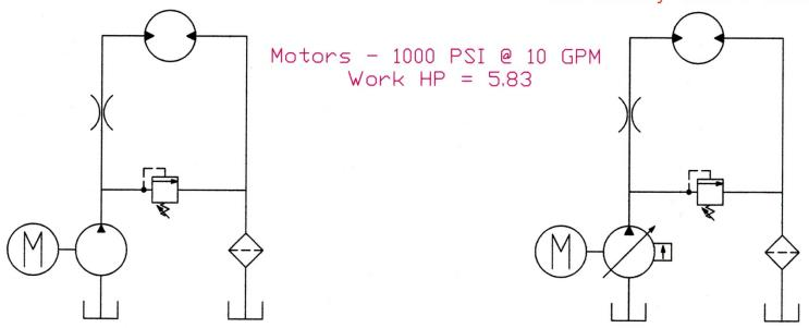
System Pressure - 3000 PSI System Max. Flow - 30 GPM
