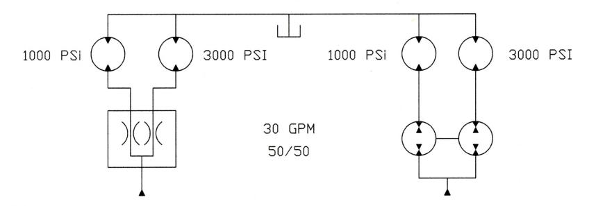
Required system pressure is 3000 PSI. Pressure drop across left side of flow control is 2000 PSI. Loss energy is 2000 x 15 / 1714 =
