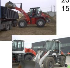
2001 DC wheel loader prototype @ TUHH with O&K 15% less fuel measured in comparison test
