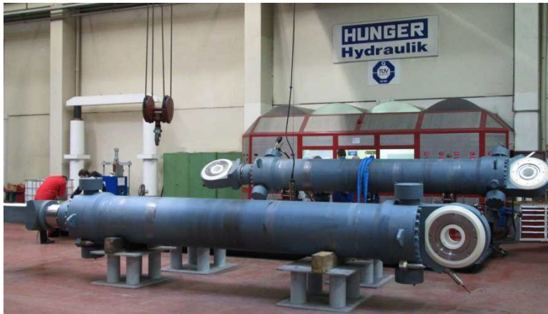
Figure 07: Oyster 800 cylinders on the hydraulic test rig
