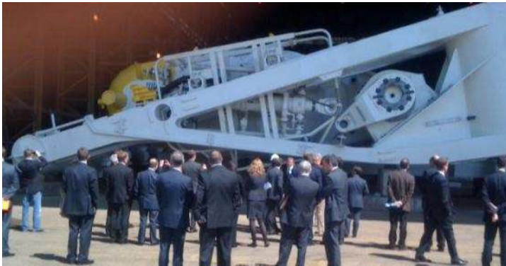
Figure 04: The cylinder module within Oyster 800
