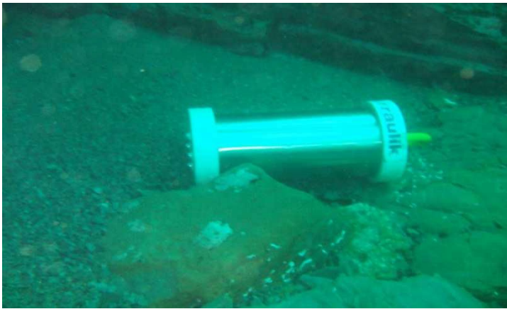
Figure 09: Test piece with Ultraplate layer in the North Sea
